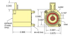
Normally Closed 2- & 3-Way Electronic Poppet Valves with Top Pin Connector
